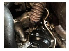
Remove bolts (4) and detach exhaust gas recirculation pipes Use the new gaskets provided on reassembly
